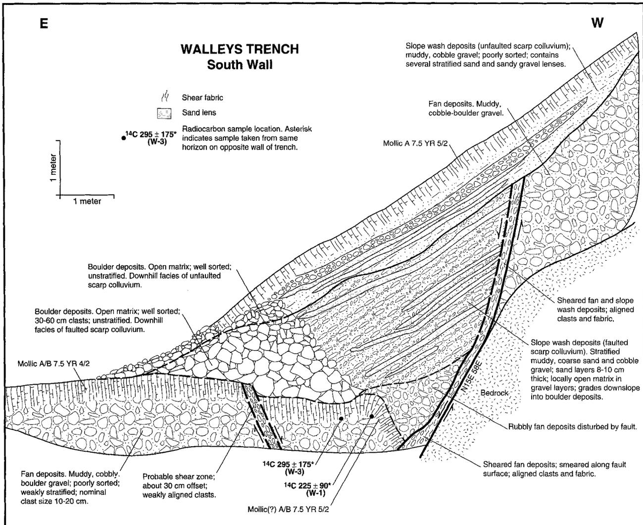
Figure 8. Log of the Walleys trench, located on the lower and smaller of two uplifted terraces near Walleys Hot Springs (Fig. 7). The trench exposed fan deposits displaced by more than 8 m during two events. Two charcoal samples yielded anomalous modern ages and are thus disregarded.
