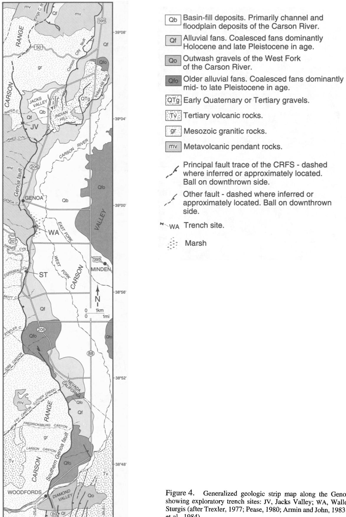
Figure 4. Generalized geologic strip map along the Genoa fault, showing exploratory trench sites: JV, Jacks Valley; WA, Walleys; ST, Sturgis (after Trexler, 1977; Pease, 1980; Armin and John, 1983; Armin et al., 1984).
