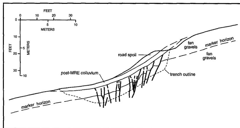
Figure 6. Simplified cross section at the Jacks Valley trench site based on trench relations and an adjacent surveyed topographic profile. Consistent stratigraphic position of a marker horizon (strongest charcoal layer) indicates that the trench exposed alluvial fan deposits displaced by more than 5 m during the most recent event.
